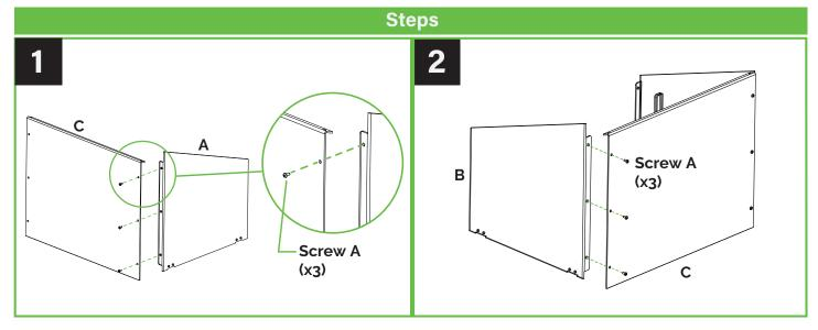
Screw Part A into Part C using Screw A (x3). Ensure that Part C is sitting on top.
