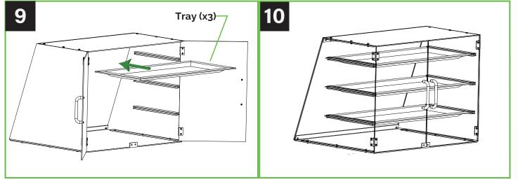
Slide in Tray (x1) into the first slot to make sure it slides in smoothly. Next, slide in the remaining Trays (x2)
