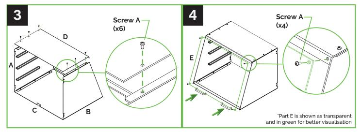
Flip the unit with Part C sitting on the base. Sit Part D on the edges of both Part A and Part B. Fix in place with Screw A (x6).
